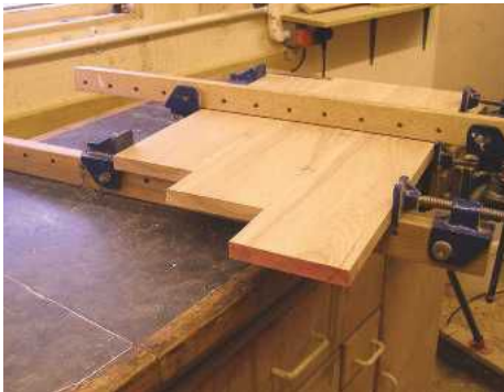
▲ Pic.3 Clamp the boards together, applying the clamps above and below to even out the clamping forces
